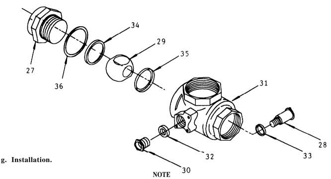
Be sure to wrap tape in same direction as pipe thread.
