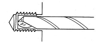
(b) Drill three quarters way deep into broken stud or screw using an appropriate size drill bit.
