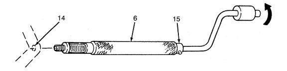
(16) Turn handle of insertion tool (6) to the left until insertion tool can be removed.
