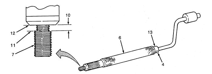
(13) Turn handle until tang of insert (7) is even with tip of insertion tool (6).
