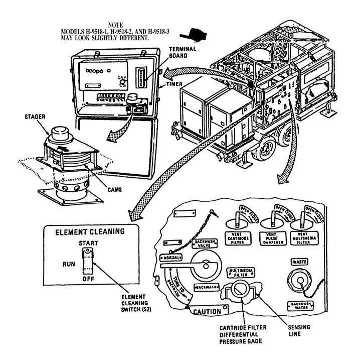
Step 3. Check for clogged control tubes. Refer to Paragraph 2-68 for routing of tubes.
