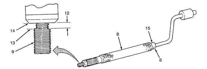
(18) Turn handle until tang of insert (9) is even with tip of insertion tool (8).
