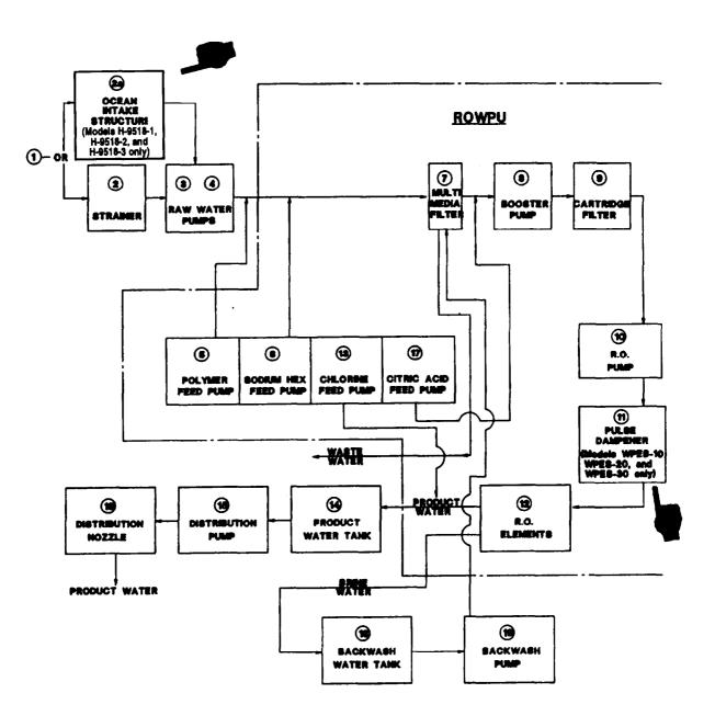
Figure 1-5. Water Processing Diagram.
