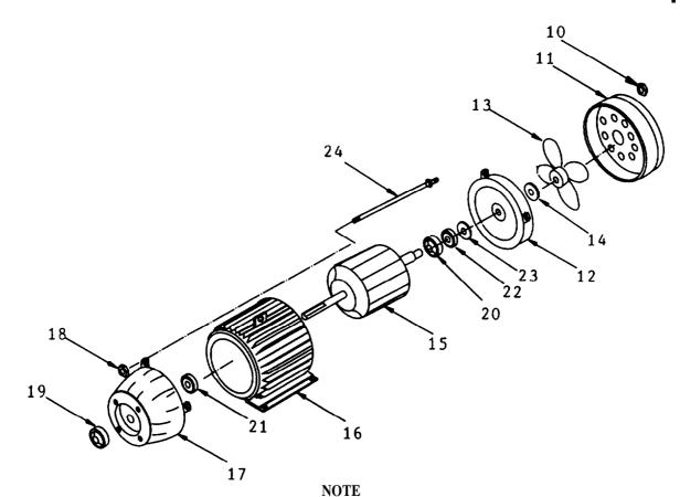
Marking relative position of casing and brackets will facilitate installation. Be sure to transcribe markings to replacement parts if defective parts are to be discarded or turned in to Supply.
