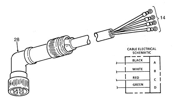
(3) Using multimeter, test for internal short between plug (28) pins as follows:
