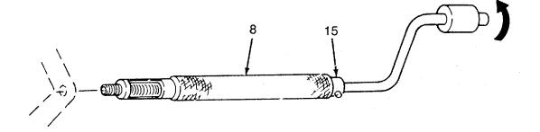
(21) Turn handle of insertion tool (8) to the left until insertion tool can be removed.
